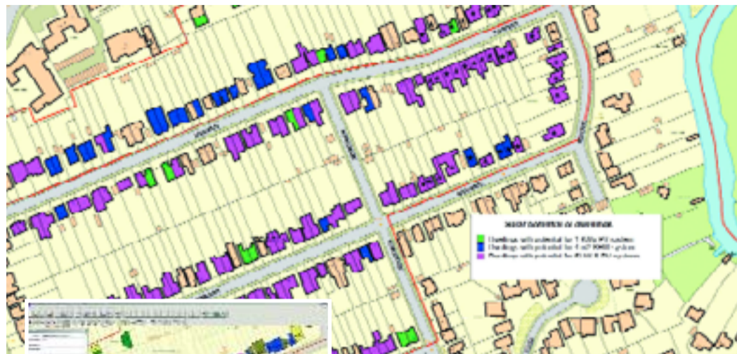
DECoRuM uses GIS software, MapInfo, to extract input data for the underlying energy models and display results in the form of colour-coded thematic maps with an individual dwelling displayed as the basic unit of resolution (Figure 1 - top)
